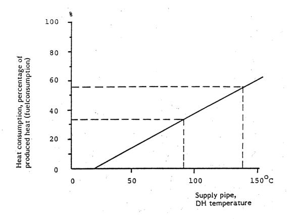
Fig. 4. The increase of fuel consumption as a function of CHP-extraction temperature
